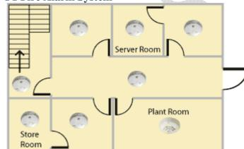
The system is installed throughout the building - the objective being to call the fire brigade as early as possible to ensure that any damage caused by fire is minimised. Small low risk areas can be excepted, such as toilets and cupboards less than 1m<sup>2</sup>.
