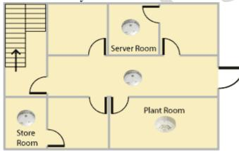
Detection should be provided in parts of the building where the risk of ignition is high and/or the contents are particularly valuable. Category 2 systems provide fire detection in specified parts of the building where there is either high risk or where business disruption must be minimised.
