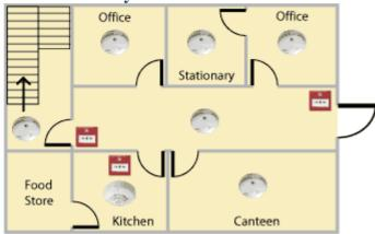
A category L2 system designed for the protection of life, which has automatic detectors installed in escape routes, rooms adjoining escape routes and high hazard rooms. In a medium sized premises (sleeping no more than ten residents) a category L2 system is ideal. These fire alarm systems are identical to an L3 system but with additional detection in an area where there is a high chance of ignition (e.g. kitchen) or where the risk to people is particularly increased (e.g. sleeping risk).
