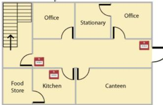
Manual systems e.g. hand bells, gongs etc, may be purely manual or manual electric, the latter may have call points and sounders. They rely on the occupants of the building discovering the fire and acting to warn others by operating the system. Such systems form the basic requirement for places of employment with no sleeping risk.
