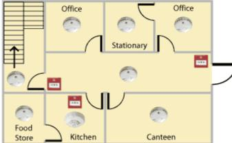
A category L1 system is designed for the protection of life, which has automatic detectors installed throughout all areas of the building (including roof spaces and voids) with the aim of providing the earliest possible warning. A Category L1 system is likely to be appropriate for the majority of residential care premises. In practice, detectors should be placed in nearly all spaces and voids. With category 1 systems, the whole of a building is covered apart from minor exceptions.
